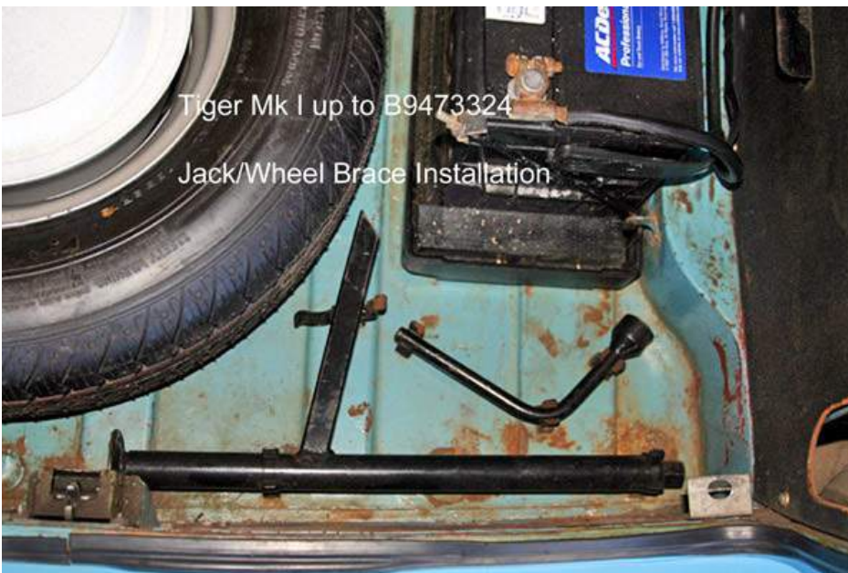
The arrangement of the short Jack and Wheel Brace in a Mk 1
